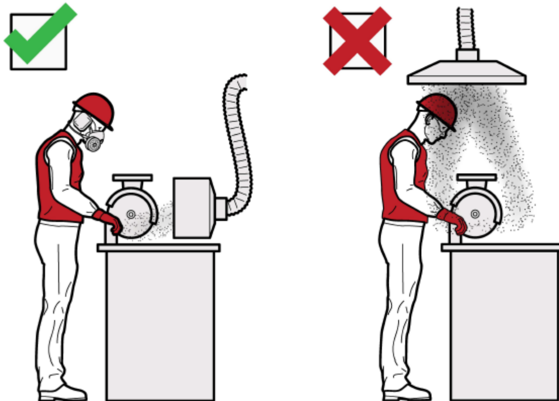
Figure 7 Examples of using local exhaust ventilation
